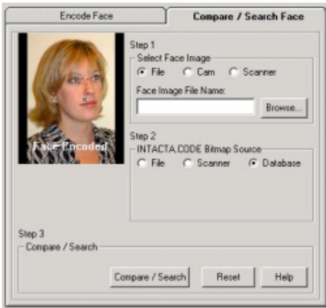
At the left is a screen shot of Xpress ID 2000, an Intacta product that encodes facial recognition data for storage in a data base or for printing on an ID card. When the ID card is scanned, the data can be compared to a data base or the individual in possession of the ID card.
