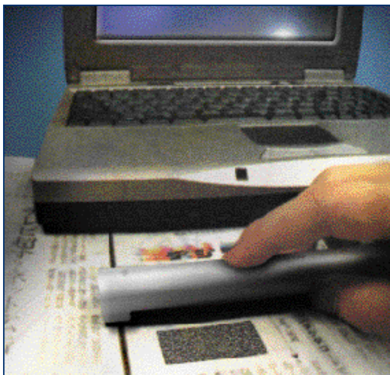
Pen Scanner reads INTACTA.CODE™
